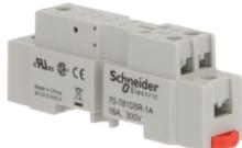
Socket, General Purpose Relays, for 781 relays, SPDT, 5 pins, screws clamp terminals, 16A, 300V
